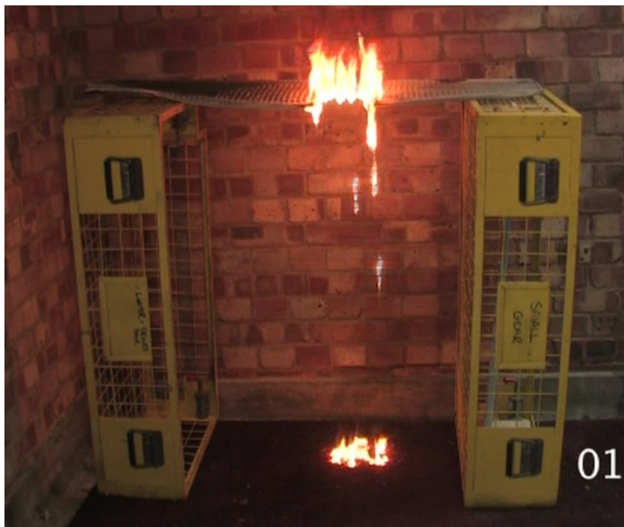
Photo 8 – Test Burn 1 Flaming molten droplets
